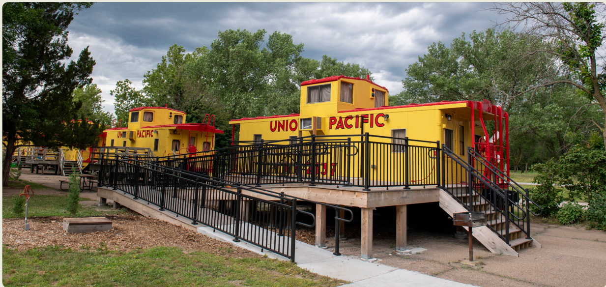
Ten cabooses that once served Union Pacific Railroad are furnished as cabins at Two Rivers State Recreation Area in Douglas County. Improvements completed in 2022 through the Capital Maintenance Fund include making one of the cabooses American with Disabilities Act compliant; it now has a wheelchair ramp, a wider door and renovated bathroom (see photo next page). All cabooses also got a fresh coat of paint. ERIC FOWLER, NEBRASKALAND
