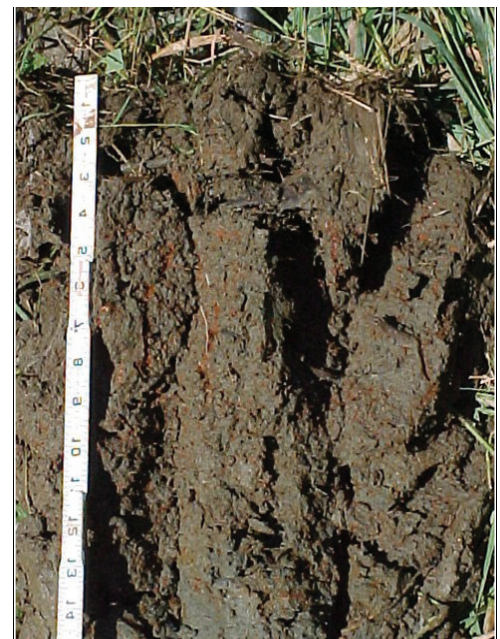
Figure 5. Redox Concentrations (reddish patches) in a prairie hydric soil. Source: North Dakota NRCS
